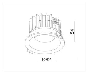
Downlight with reflector and protection glass, in a high quality matt finish, suitable for a variety of residential applications as well as in restaurants, hotels or bars.
