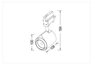
Alliance Track lights have a very compact design thanks to their built-in driver. They are therefore less disturbing when they are used in retail spaces, shop windows or showrooms. However, the light performance is their greatest asset. The optical lens ensures an optimum light beam and very low glare.
